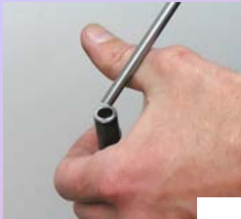
Inserting of the punch wire into the probe.
