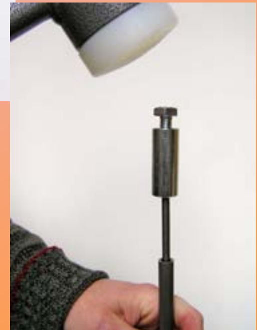
Screwing the distance screw till it touches the distance ring.
