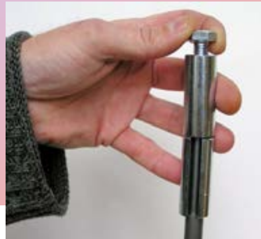
Screwing the distance screw till it touches the distance ring.
