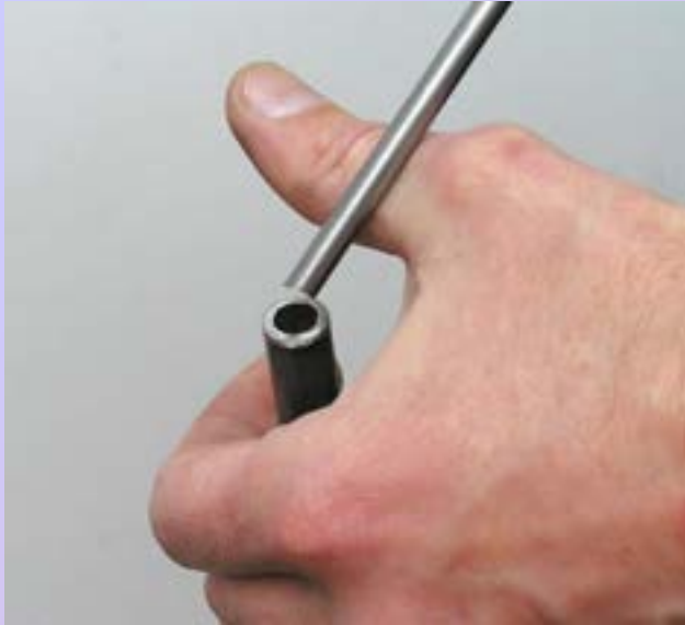
Step 5: Inserting of the punch wire into the probe.
