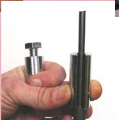
Inserting of the distance ring.
