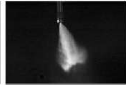
I-Injector (Single Hole Injector, Inward Opening, With Swirl Component)
