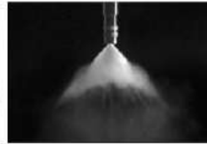
O-Injector (Pintle Injector, Outward Opening)
