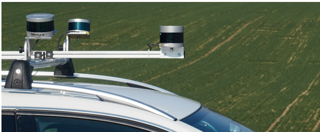
Fig. 6. Velodyne VLP-32 mounted on the experimental vehicle. Only the Velodyne VLP-32 in the front was used for this paper.
