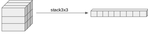
Fig. 7. Illustration of the stack3x3 operation. It may be thought of as a convolution operation with binary weights (0 or 1) such that each output pixel is a concatenation of neighbouring pixels in the input.
