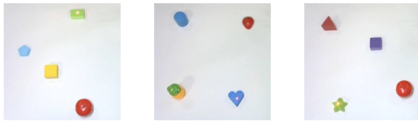
Fig. 16. Specular highlights on some of the objects appear similar to the laser pointer and cause poor performance
