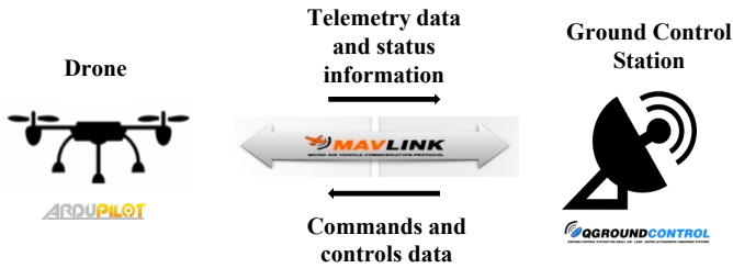
Fig. 1. Communication link between UAV and GCS.
