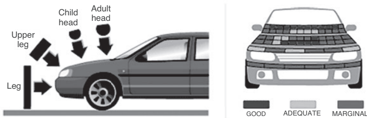
Figure 1.1e Pedestrian impact tests
