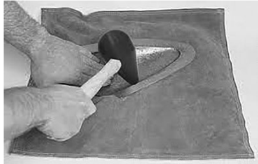
Figure 3.2 Body mallet in use
