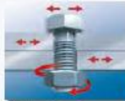
Vibration and loosening
