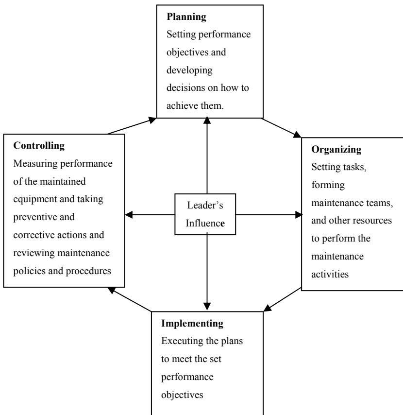
Figure 5.2. Maintenance control as a function of the management process
