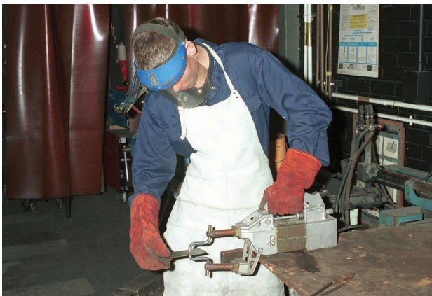
Figure 2.2 Protective clothing for spot welding
