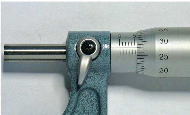
Figure 4.19 Metric system – micrometer thimble reading 5.78mm
