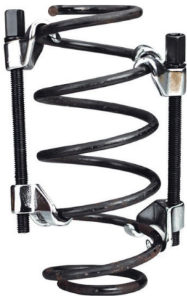
Figure 4.33 MacPherson springs must be compressed for removal
