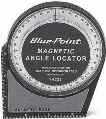
Figure 4.23 This device checks propshaft angles
