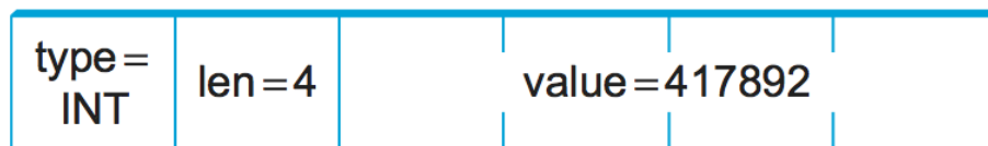
A 32-bit integer encoded in a tagged message.
