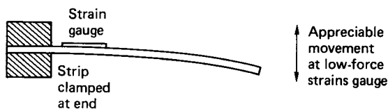
FIGURE 6.34 Strain gauge on flexible strip.
