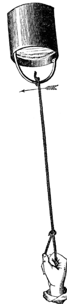
Figure 23.2: A bucket of water being spun in a vertical circle. Inertia (sometimes thought of as a fictitious “centrifugal force”) keeps the water in the bucket, even when upside-down. (Ref. [20]).
