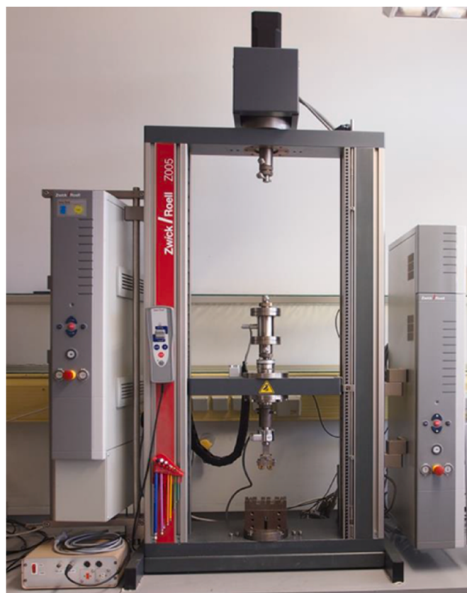
Fig. 6. Universal testing machine (Zwick/Roell Z-005, Zwick/Roell S.L.).
