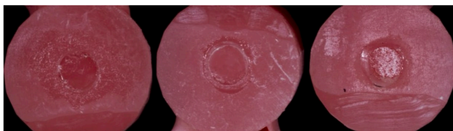
Fig. 4. Type of bond failure: Cohesive (left), adhesive (centre) and mixed (right), measured under a stereomicroscope.
