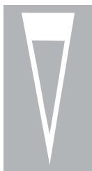
Warning of “Give Way” just ahead
