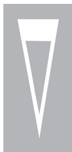
Warning of "Give Way" just ahead
