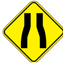
Pavement narrows ahead
