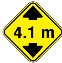
Low structure clearance 4.1 metres
